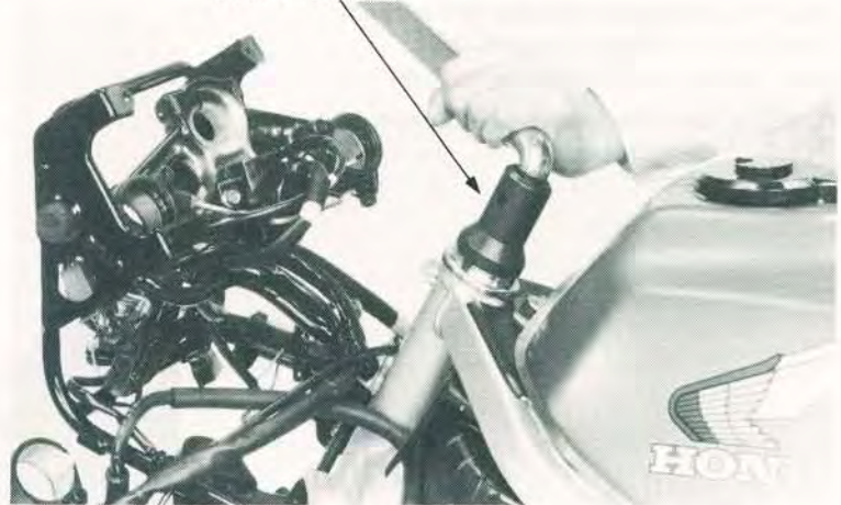
STEERING STEM SOCKET 07916–3710100
