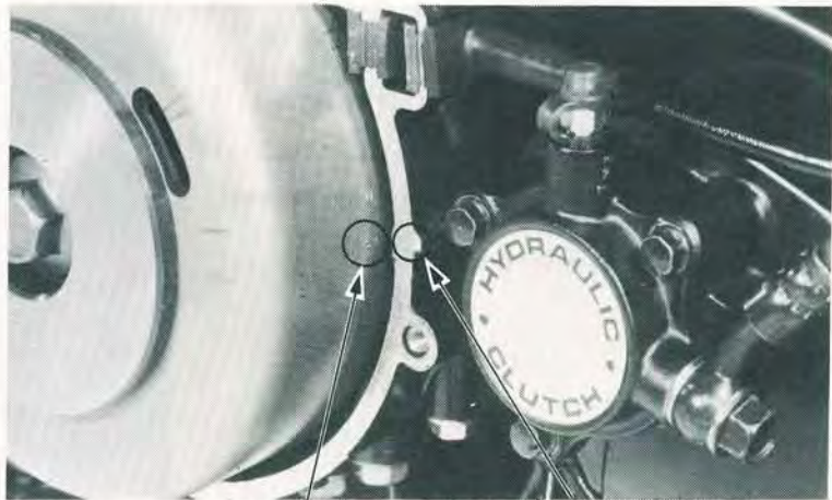
T1.3 MARK REAR MATING SURFACE
