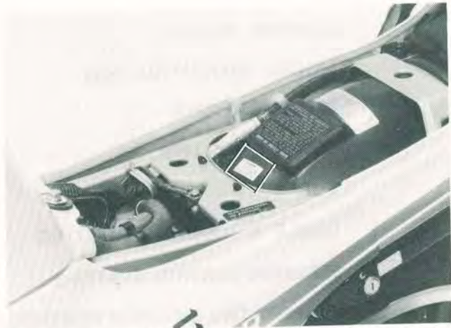
The color label is affixed to the rear fender, under the seat.
