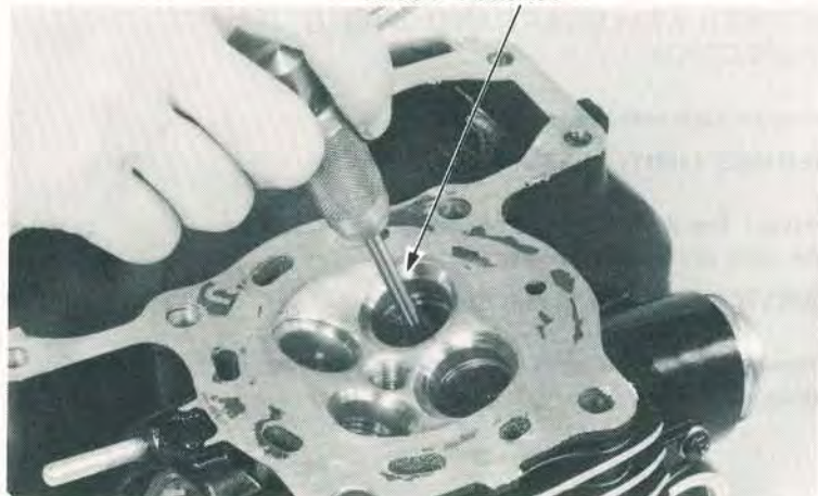
VALVE GUIDE REAMER 07984-2000000
