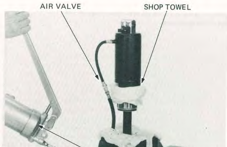
GREASE GAN FILLED WITH ATF
