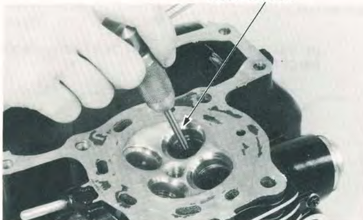
VALVE GUIDE REAMER 07984-2000000
